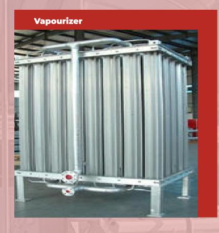
The fins absorb the warm ambient air and transfer the heat to the cryogenic liquid flowing in the tube. The heat transfer converts the liquid into a gas. Ice accumulations on these systems are normal
